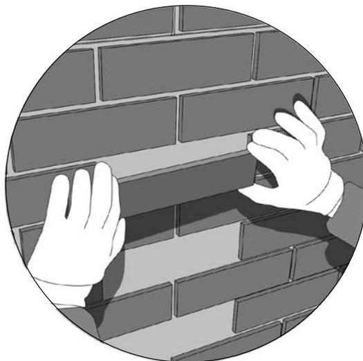
**6.3.** Check that surfaces of the tiles to be pasted are aligned exactly to the surface plane of pebble-dash panels and are at the same height.
